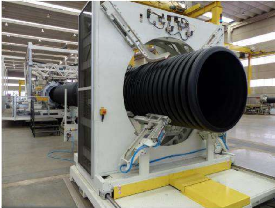
Figura 1 - Fabricación del Tubo KNTS Drain / Figure 1 – KNTS Drain Pipe Manufacturing Process
